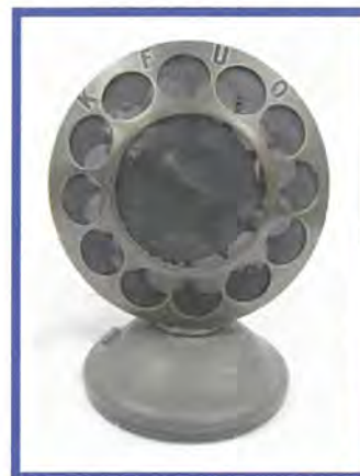
From the CHI collection: the Western Electric double-button spring-suspension carbon microphone (1920s) used in the earliest days of KFUD radio.
